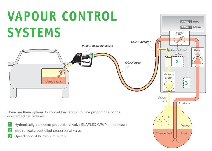
At the heart of the vapour recovery system is the device used to control the volume of vapour recovered relative to the liquid dispensed. Both have to correspond. To achieve the correct ratio, it is necessary to control the vapour volume flow.
