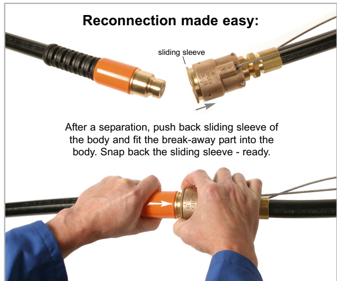
ARK 19 Mod. 2: Easy reassembly on site, under pressure.
