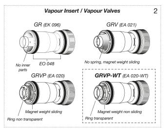
The **GRVP-WT** (EA 020-WT) is supplied ready for installation, pre-adjusted and tested for vapour tightness. Only the O-rings are supplied as spare parts. In the case of a malfunction the whole GRVP-WT unit is to be replaced.
