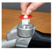
Remove diaphragm spring EF 250.2, diaphragm assembly EA 151.
