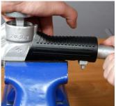
tool EW 3 into diapgragm chamber to secure pull rod assembly EA 058.
