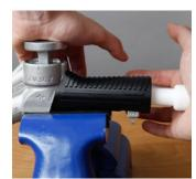
Use assembling tool EW 5-3 to push the pull rod assembly EA 058 inside, against the force of the main spring.
