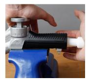
Push EW 5-3 into nozzle body and compress main spring. Put EW 3 into diaphragm chamber to fix EA 058.1
