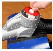
Clamp the nozzle tilted into the vice. With rollers showing downside insert diaphragm assembly EA 151 into diaphragm chamber.
