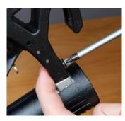
Insert rear screw EB 278 and tighten it with a torque of 3 Nm (hand-tight).
