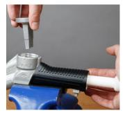
Remove assembling tool EW 3 from the diaphragm chamber. Release spring tension by removing EW 5-3.
