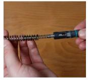
Oil pull rod assembly EA 058.1 thoroughly. Push return spring EF 064.1 with main spring EF 060.1 onto pull rod assembly.
