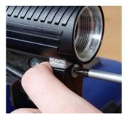
Unscrew guard screw assembly EB 438 with two screwdrivers EW 669/2 and rear screw assembly EB 278.
