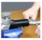
Screw it in with EW 3. Remove assembling tools.
