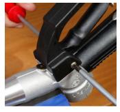
Tighten screws with screwdrivers EW 669/2.
