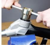
Apply oil on nozzle thread, o-ring zone and outer border of the diaphragm. Screw vacuum cap EK 148.1 or EA 052 (DSA) hand-tight into the nozzle body.
