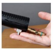
Tilt nozzle body and remove pull rod assembly EA 058, main spring EF 060 or EF 061 and return spring EF 064.
