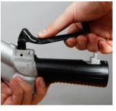
Oil lever bolt and insert lever EA 030 into nozzle body.
