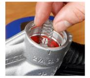
Squeeze lever to check that rollers are engaged into pull rod assembly. If ok, position diaphragm spring EF 250.2 centred on the diaphragm assembly.
