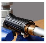
Remove valve seat EG 069 / 068 with double box spanner EW 19/22.
