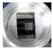
Check alignment of pull rod assembly recess. It should show upwards.
