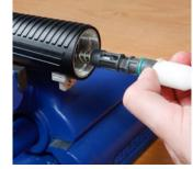
Push this group onto assembling tool EW 5-3, oil it and insert it as shown into the nozzle body.
