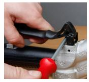
Lift up lever assembly EA 030 by levering with a screwdriver.
