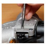
On both sides pull out lever pins EB 235 with EW 2 CV.
