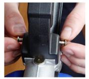
Insert guard screw assembly EB 438.
