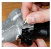
Align lever to the holes in the nozzle body. On both sides insert lever pins EB 235 to secure lever.
