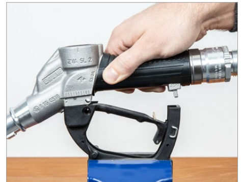
Separe el cuerpo de la pistola y la manija. Asegure de que los pasadores de palanca EB 235 no se caigan. Pull off the nozzle body and remove guard from the vice. Make sure that the lever pins EB 235 do not fall out.
