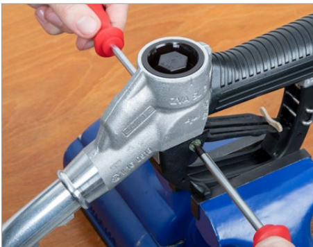
Afloje los tornillos protectores EB 438.1 con los destornilladores. Unscrew guard screw EB 438.1 with screwdrivers.
